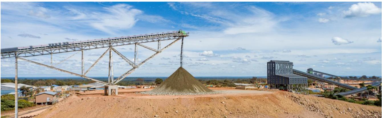
Kakula's main pre-production stockpiles at the northern declines. The blended stockpiles currently contain approximately **1.64 million tonnes grading 4.93% copper**. The run-of-mine stockpile in the previous picture is circled in red.
